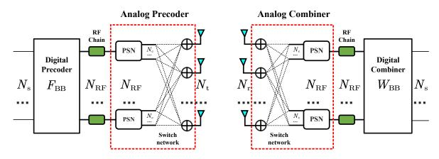
Fig. 1. A point-to-point mmWave massive MIMO system with the FPS/VPS architecture.
