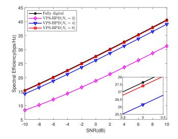
Fig. 3. SE comparisons of the VPS-HPD scheme with different  $N_{\rm c}$ .
