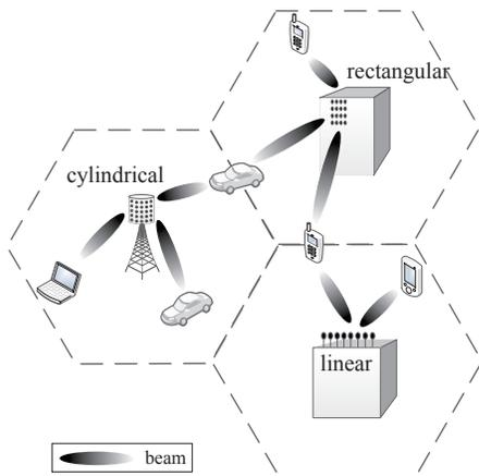
Fig. 1. Three different configuration of BS antennas in massive MIMO systems.
