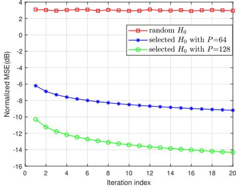
Fig. 2. Convergence of the initial channel estimation algorithm.
