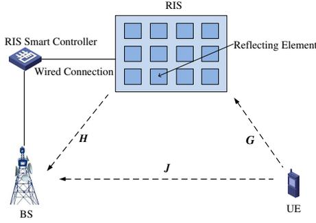
Fig. 1. Illustration of RIS aided MIMO wireless communication system.
