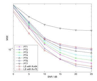
Fig. 3. MSE performance comparisons of channel estimation for different pilot design schemes.
