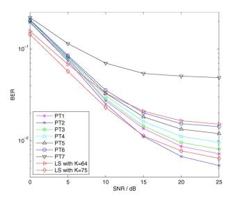
Fig. 4. BER performance comparisons of channel estimation for different pilot design schemes.
