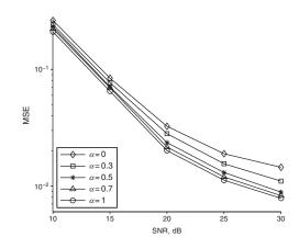
Fig. 2 Comparison of sparse channel estimation performance
