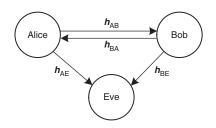
Fig. 1 Wireless communication system including two legitimate users Alice and Bob and eavesdropper Eve
