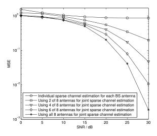
Fig. 2. Comparisons of individual sparse channel estimation and joint sparse channel estimation in terms of MSE with the fixed positions of nonzero entries of CIR.
