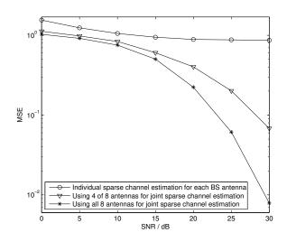
Fig. 3. Comparisons of individual sparse channel estimation and joint sparse channel estimation in terms of average MSE with random positions of nonzero entries of CIR.
