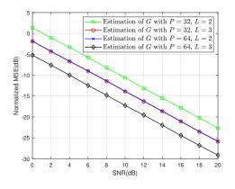
Fig. 4. Performance comparisons for regular channel estimation.
