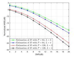
Fig. 3. Performance comparisons for initial channel estimation.
